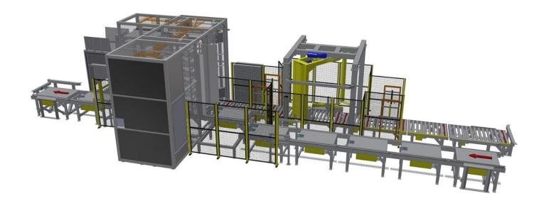
The MMC First Process Direct Palletizer is a solidly-built, high-capacity, electro-pneumatic palletizing system. There are no hydraulics, with associated spillage risks. The electrical design gives increased operational reliability and lower maintenance costs.
