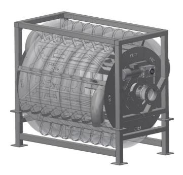
The MMC First Process RID Pumping system (Patented) is the only spiral pump system with a suction function. The pump is specially designed for transporting fish gently. Chilled water is important for maintaining good quality. The amount of water depends on the fish species.
