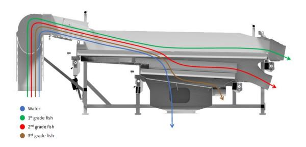
The MMC First Process duo grader for live fish consists of two layers with rollers. The D-grader comes in two sizes, D10 and D14. The roller gaps, tilt and rotation are adjusted by electric control.
