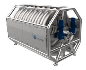
The product is gently transported in water in a closed system, Variable speed and capacity makes it possible to control the flow. The closed system makes it possible to transport products over long distances. The RID pump is chosen based on the size of the product, distance and lifting height.
