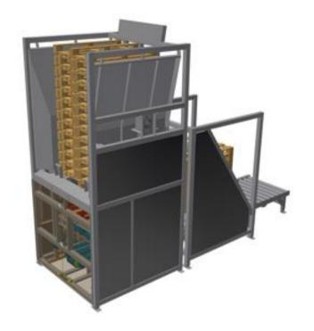
When stacks of pallets arrive at the factory, the pallets are stacked with every second one upside down, in order to save space during transport. The pallets must therefore be re-organized and re-stacked, before they can used in a seafood production line.
