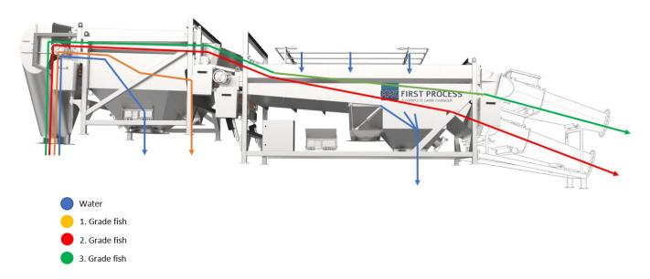
The MMC First Process T-grader is our standard grader for live fish. It consists of a pre-grader and a main grader. The T-grader comes in two sizes, T10 and T14, denoting the number of gaps. The roller gaps, tilt and rotation are adjusted by electric control.
