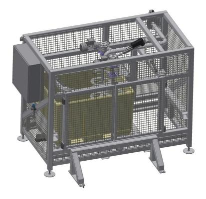
The MMC FIRST PROCESS Roe Mixer is specially constructed to handle the fragile and valuable herring roe as gently and sensitively as possible – this was a top priority during the design and development phases.
