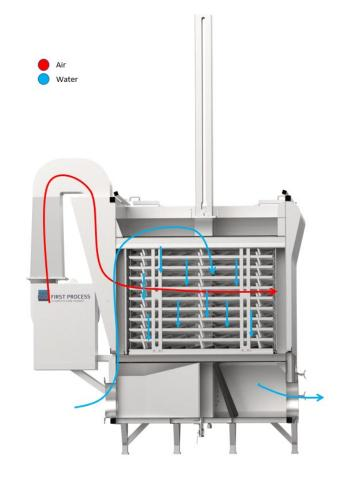
The X-AIR<sup>TM</sup> element maximizes the water surface area, and the cross flow system removes  $CO_2$  efficiently. The foam creation is minimized.
