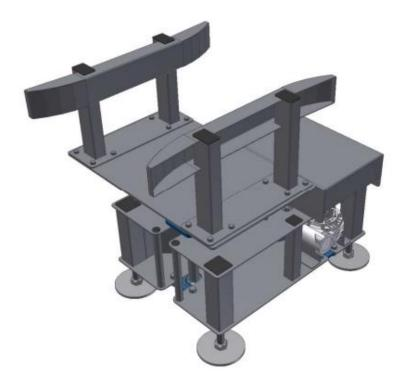
The MMC FIRST PROCESS Ice Levelling system is designed to gently level out the ice in EPS boxes containing fish. The machine shakes the box sideways, at the front and at the rear alternately. The effect is to flatten out the top surface of ice and fish in the box.
